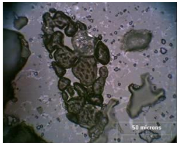
Clinker from RX B With 2% ACSS Well developed small free lime cluster along with scattered periclase in the clinker grains
